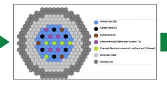
Fuel assemblies would be loaded into the VTR core during a refueling outage at the end of a test cycle. The initial core would require 66 driver fuel assemblies. Up to 15 driver fuel assemblies would be replaced 3 times a year.
